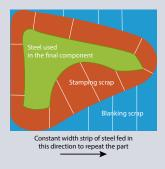
Half of all sheet steel is scrapped during manufacturing: in this example, the car panel doesn't tessellate, and extra material is needed for grip while it is shaped
