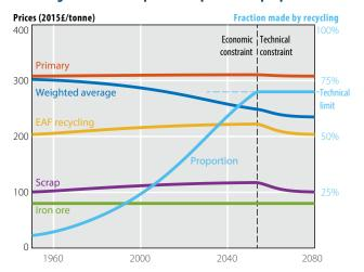
a pattern derived from the analysis on page 3. Steel made from scrap in electric arc furnaces is assumed to be a perfect substitute for steel from the primary blast furnace route up to a technical limit and the relative proportions of the two forms of production is found by cost minimisation. Cost and price data have been estimated from several sources to be approximately representative of 2014-15 but model outputs are intended more as indicators of trends than as quantitative predictions.
