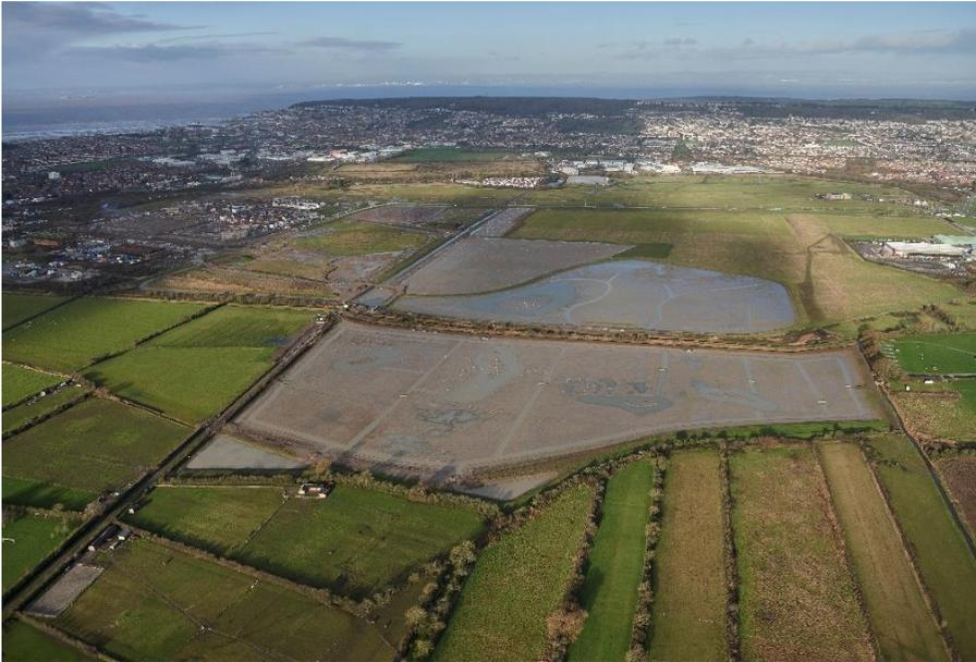
Reservoirs are where water is stored above normal ground levels. There is a slight risk that an embankment that holds the water above ground level could fail, and the water could escape and cause flooding. The management of reservoirs is heavily regulated to make sure the risk of any failure is minimal. Inspections are carried out by government appointed independent engineers.
