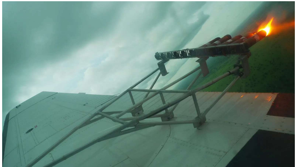
The salts are fired from a flare rack carried on the aircraft (Credit: Jean Francois Berthoumieu)
