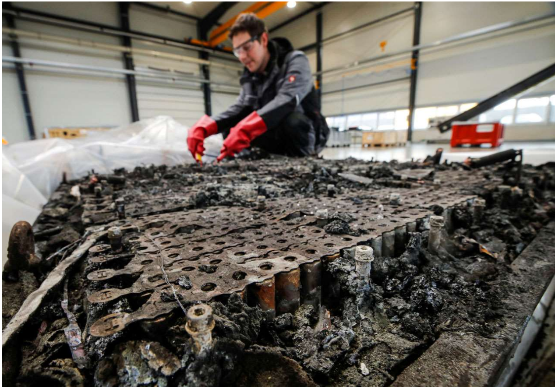
A technician in Germany makes sure a burned lithium-ion battery is discharged before further recycling. WOLFGANG RATTAY/REUTERS
