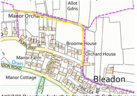
AX6/7/30 Resurface footpath to 2m wide with Selfbinda or equivalent. A semi bound surface is required due to the sloping nature of this section. Approximately 260m length by 2m wide. Shown as blue line below.
