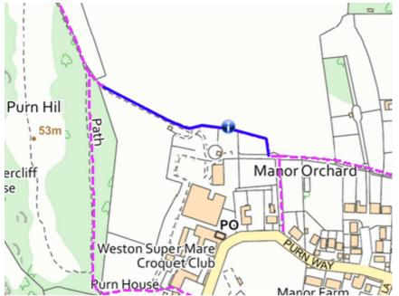
AX6/7/20 Resurface footpath to 2m width with Ultritec or equivalent. Approximately 270m length by 2m wide. Shown as blue line below.
