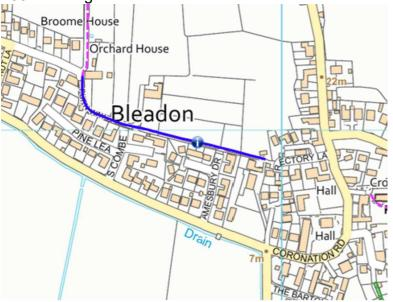
AX6/11/10 & AX6/10/20 resurface footpath to 2m wide with Tarmac Ultritec or equivalent. Approximately 400m x 2m wide. Shown as yellow line below.
