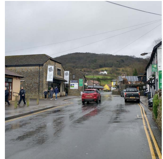
↑ Wide carriageway and absence of footway
